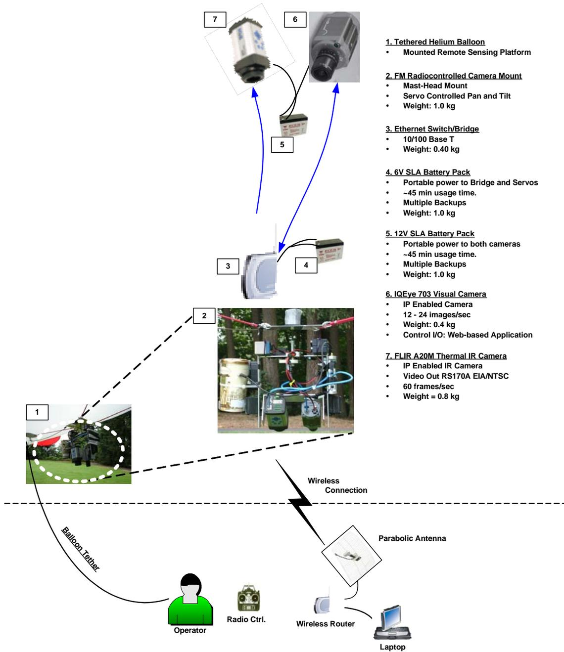
Figure 2b. Illustrative detail of remote sensing aerial platform as developed and deployed in this project. US patent Pending.
