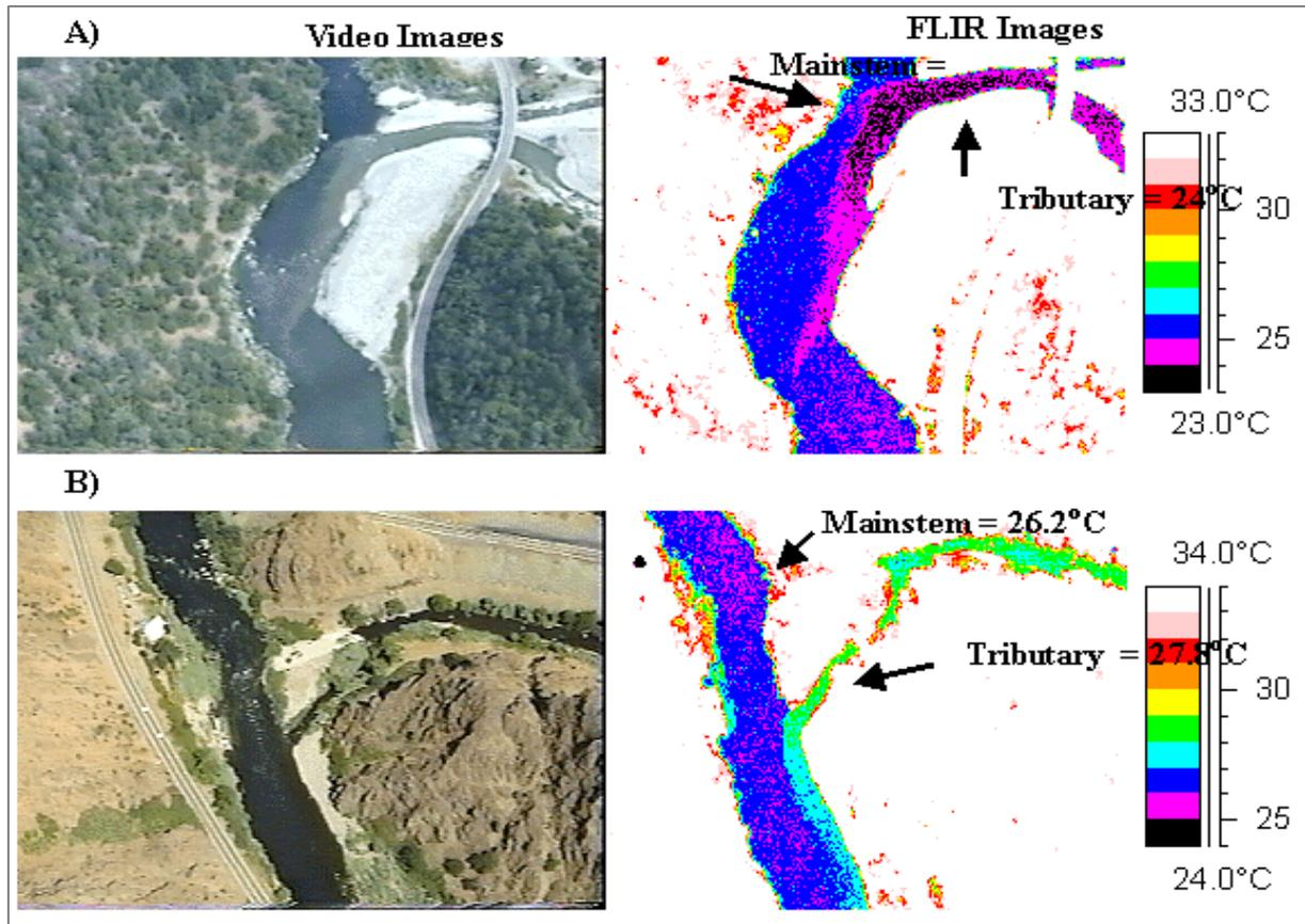
**Figure 1.** Examples of helicopter-based infrared remote sensing of mixing zones from a point source surface discharge. (Source: Oregon DEQ). Typical airborne infrared camera output consists of digital images covering approximately 100 x 100 meters with less than 1 meter of spatial resolution and  $\pm 0.5^\circ\text{C}$  accuracy. Figures A) and B) show cool and warm tributary surface discharge sources respectively. Image Source: ODEQ.
