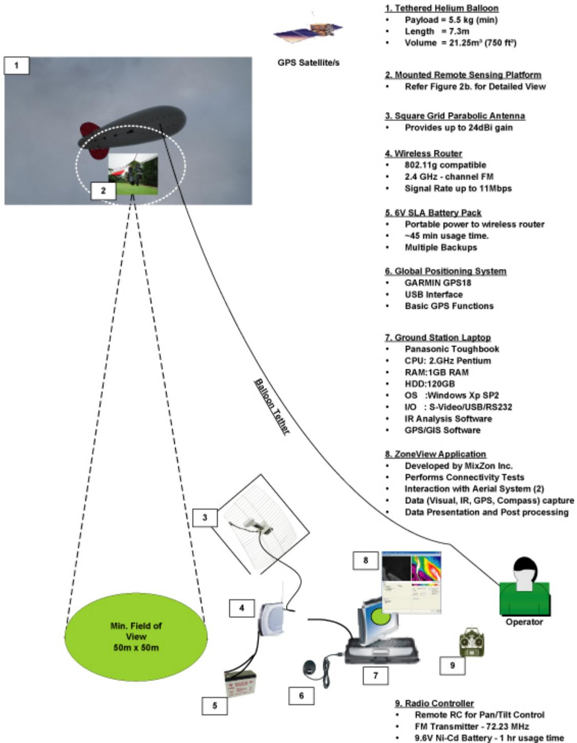
Figure 2a. Illustrative conceptual diagram of remote sensing system as developed and deployed in this project. US Patent Pending.
