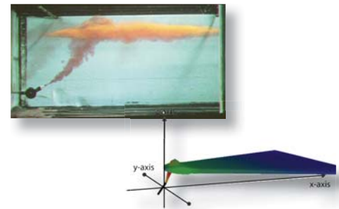
A Buoyant Jet Trapped by Density Stratification Forms a Density Current
